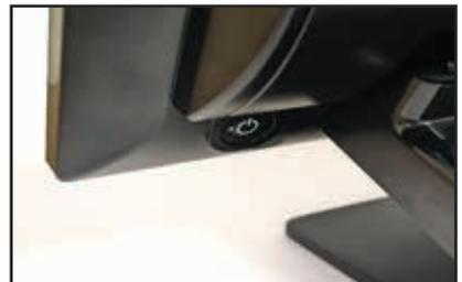
The power button for Toshiba T10 is at the bottom of the screen at the rear
